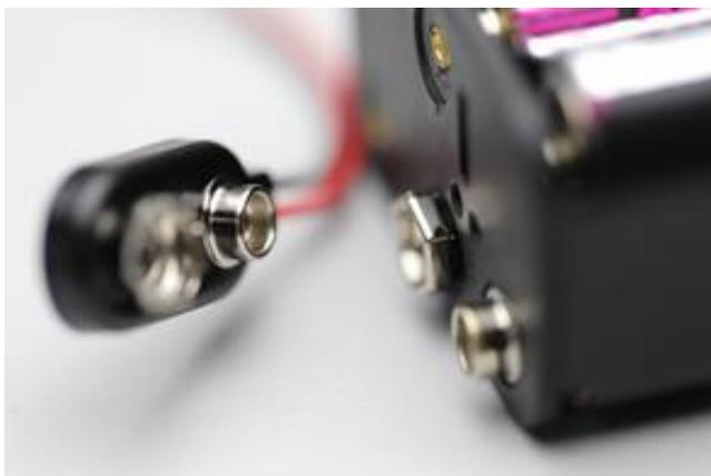
Batteriekabel an Battery Pack anbringen
